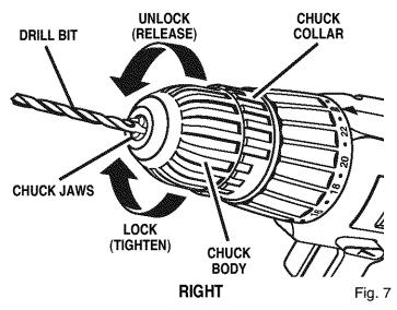
To tighten the chuck jaws on drill bit; grasp and hold the collar of the chuck with one hand, while rotating the chuck body with your other hand.
